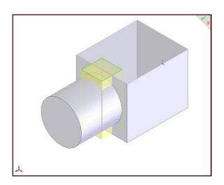
Step3: Make an extruded body for subtraction.
