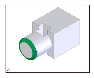
Step5: Make a fillet at the top circle edge of the main body. Radius of fillet is 1.0.
