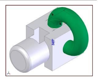
Step6: Create a sheet circle and spin it around an edge of the main body.
