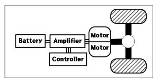
Electric Motor and wheel model
