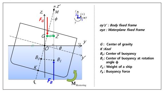
M: For a ship in upright position, the line of action of the buoyant force before inclination is the centerline, which is denoted by dot-point line. The new line of action of the buoyant force after inclination passes through the changed center of buoyancy  $B_1$  and is perpendicular to the waterplane. The two lines intersect in the point M, called metacenter.
