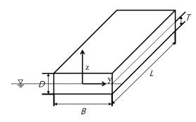
*L*=40m, *B*=10m, *D*=10m, *T*=5m Density of sea water:  $\rho \approx 1 \text{Mg/m}^3$ Damping coefficient:  $c = 4.8 \text{MN} \cdot \text{s/m}$ Added mass  $m_{added}$  is same as the mass of the ship. The ship is in static equilibrium state at z=0
