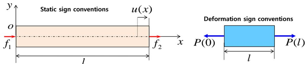
$f_1, f_2$  : Nodal forces acting on the ends of the bar element
