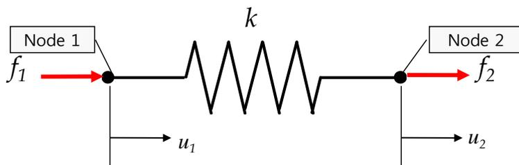
$f_1, f_2$  : Nodal forces acting on the ends of the bar element
