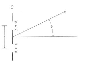
(1) Calculate the irradiance distribution of the Fraunhoffer diffraction pattern by a double-slit aperture.
