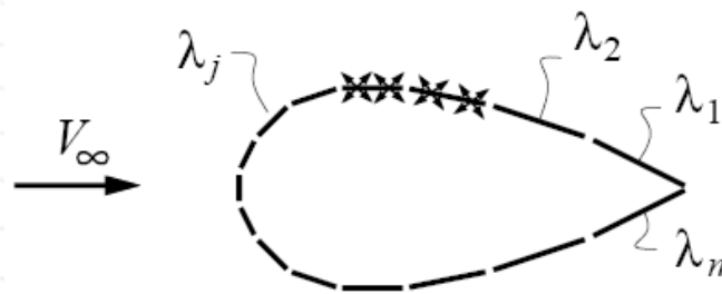
uniform flow + n source panels
