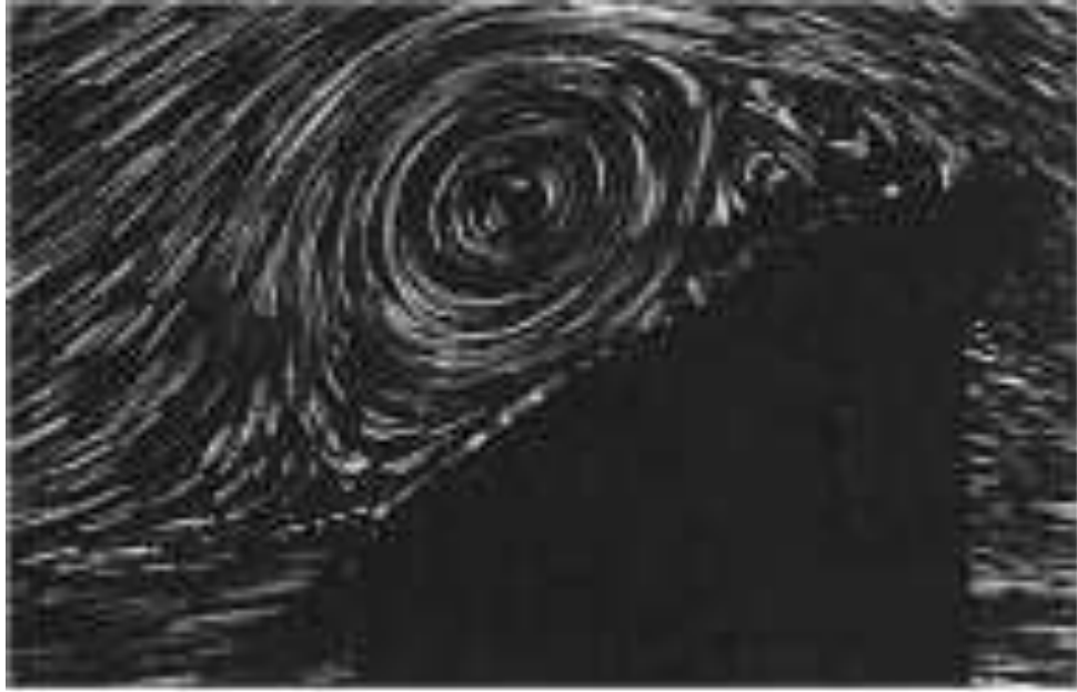
(a) Streamlines from experiment, Huang et al (2001), t = 2.348
