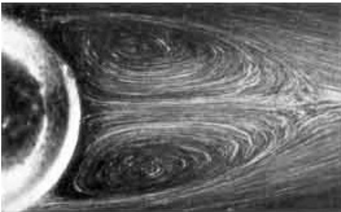
(b) Visualization from experiment ( Re = 118 ), Taneda
