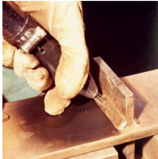
Needle peening fillet weld toe
