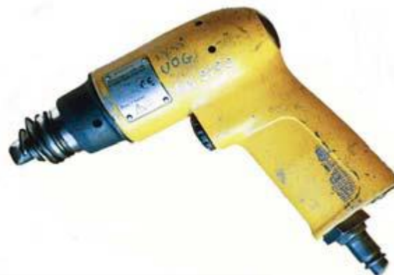
Pneumatic riveting guns used for hammer peening.
