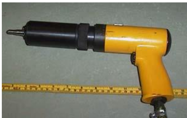
Pneumatic riveting guns used for hammer peening.
