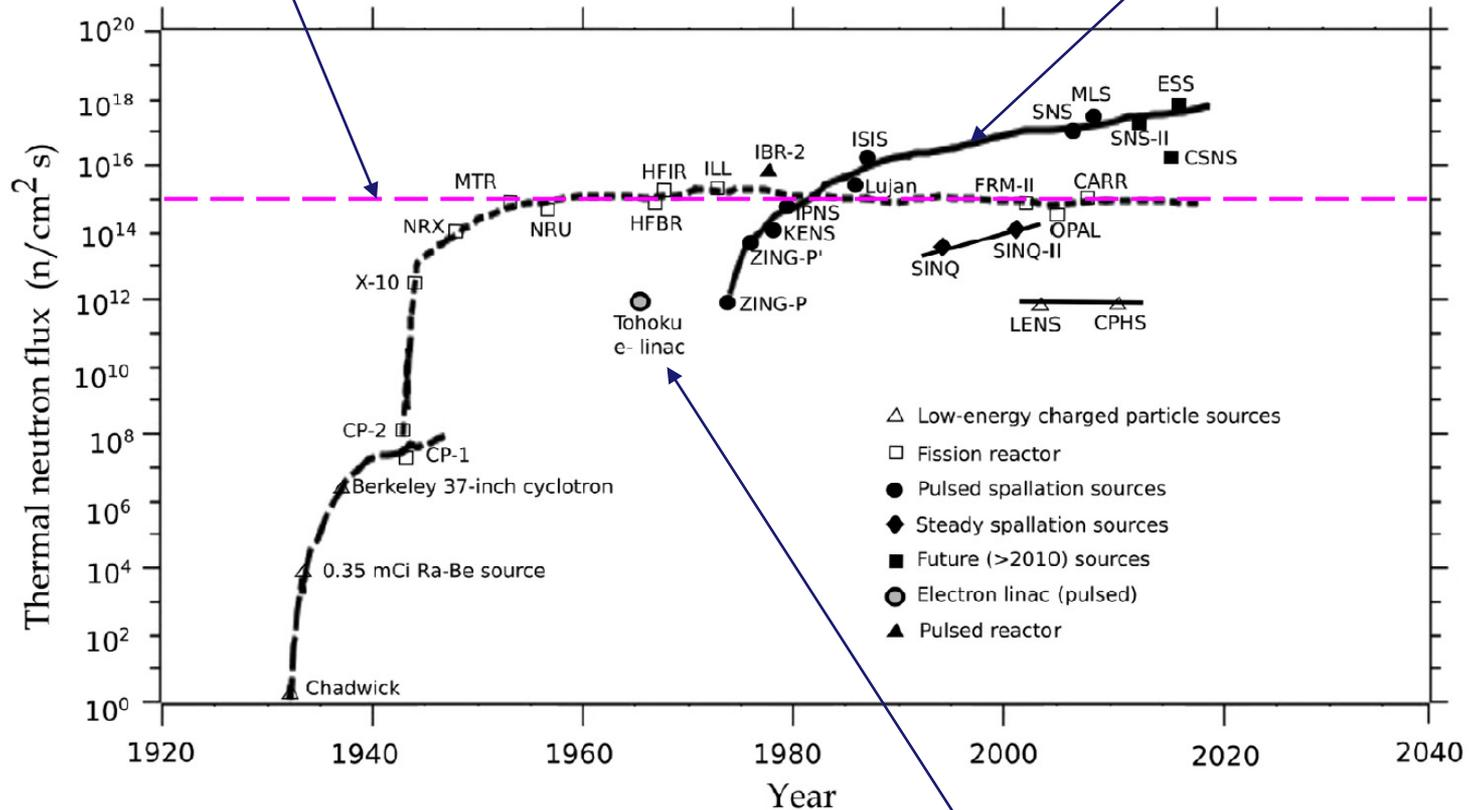
Electron-linac-driven photoneutron source (~2000 MeV / neutron)
