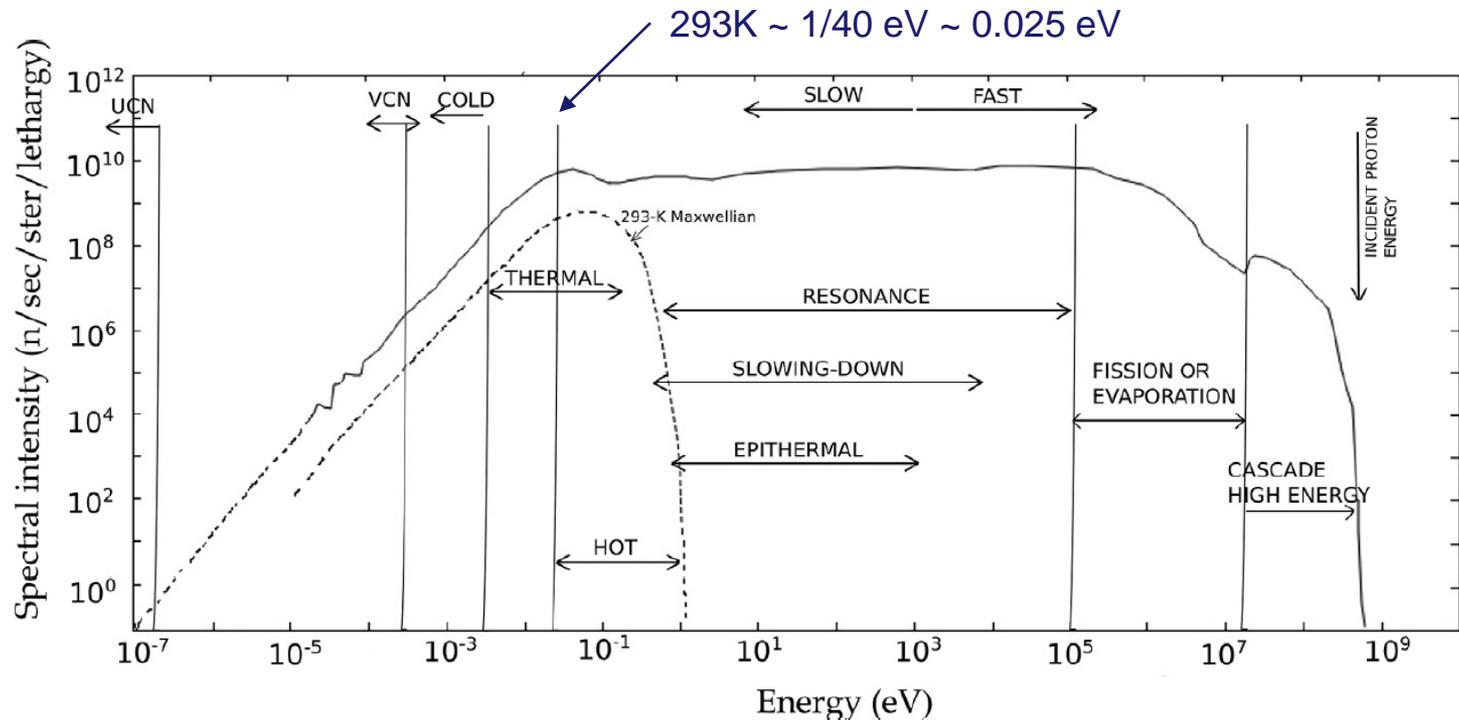
The expected neutron spectrum emitted from a 100 K liquid methane moderator of the Intense Pulsed Neutron Source (IPNS) at Argonne National Laboratory (ANL)
