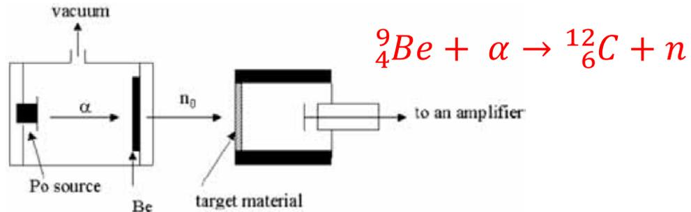
Chadwick's apparatus: 1<sup>st</sup> neutron generator
