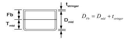
\* Freeboard (Fb) means the distance between the water surface and the top of the deck at the side (at the deck line). It includes the thickness of freeboard deck plating.
