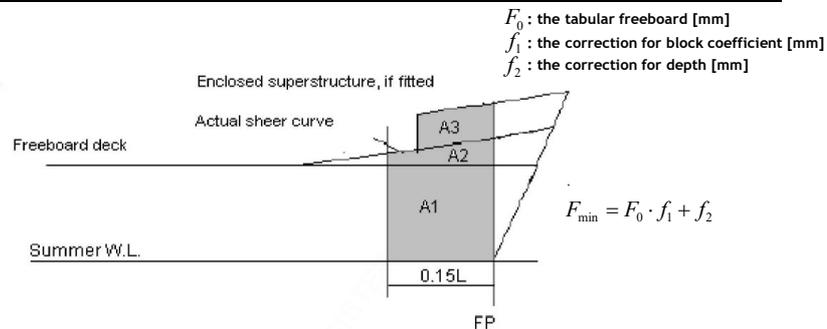
All ships assigned a type 'B' freeboard, other than oil tankers\*, chemical tankers\* and gas carriers\*, shall have additional reserve buoyancy in the fore end.
