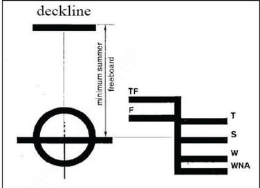
The Plimsoll<sup>1)</sup> mark or Freeboard Mark is a symbol indicating the of the ship in the water, leaving a minimal freeboard for safety. The freeboard is marked according to the result of the freeboard calculation, where the summer freeboard in salt water ( $d_s$ ) is established.
