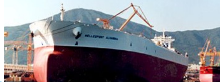
442,000ton DWT ULCC(Ultra Large Crude Oil Carrier)
