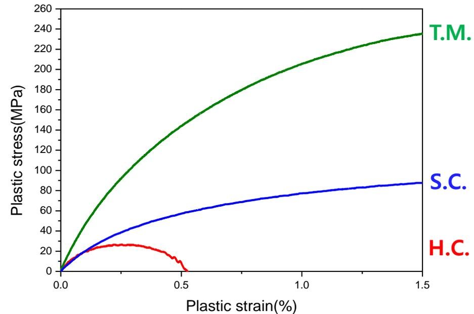
Higher strain hardening of T.M., then larger work hardenability of BMGMCs
