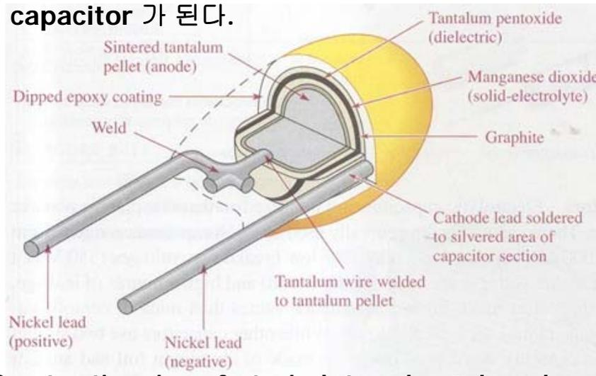
Construction view of a typical "tear drop" shaped tantalum electrolytic capacitor
