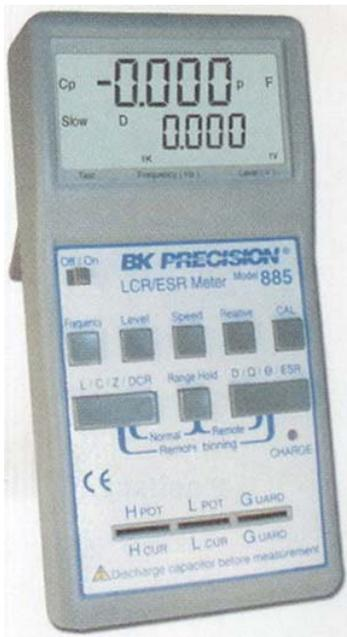
Digital reading capacitance meter.
