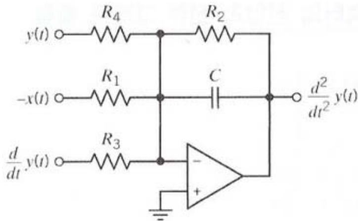
$$\frac{1}{R_1 C} = 3, \quad \frac{1}{R_2 C} = 2.5, \quad \frac{1}{R_3 C} = 2, \quad \frac{1}{R_4 C} = 1.5$$
