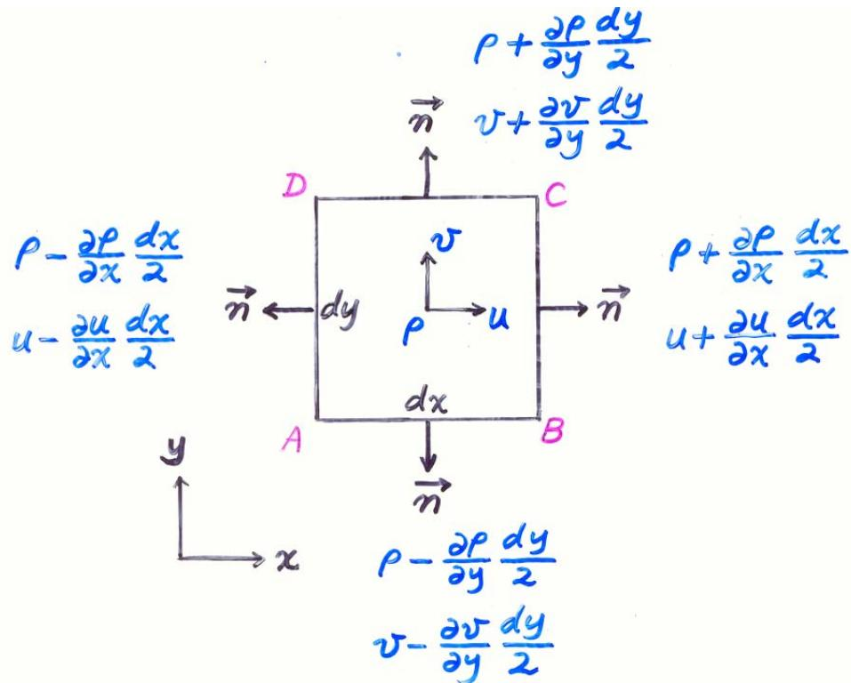
$$\iint_{ABCPDA} \rho \vec{v} \cdot \vec{n} dA = 0 \rightarrow \boxed{\frac{\partial}{\partial x}(\rho u) + \frac{\partial}{\partial y}(\rho v) = 0}$$
