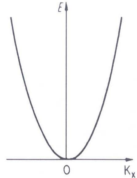
Figure 5.1. Electron energy E versus the wave vector k_x for free electrons.
