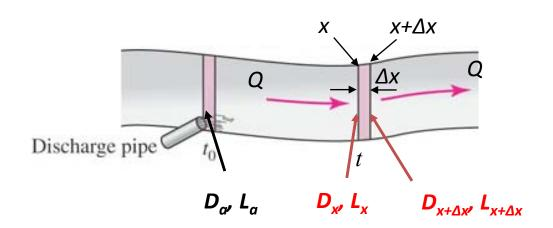
Steady-state D (= $DO_s$ -DO) balance for a thin plate at time t:
