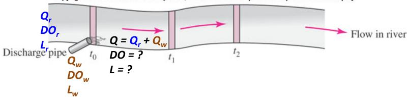
We will model the DO of a river receiving waste at time  $t_0$ . The river will be modeled as a PFR.
