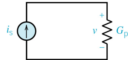
Figure 3.4-3 (p. 69) Equivalent circuit for a parallel circuit.
