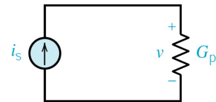
Figure 3.4-3 (p. 67) Equivalent circuit for a parallel circuit.
