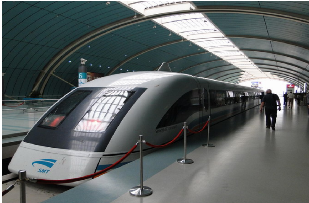
Magnetic levitation train (Maglev train, Shanghai) Floating on strong superconducting magnets
