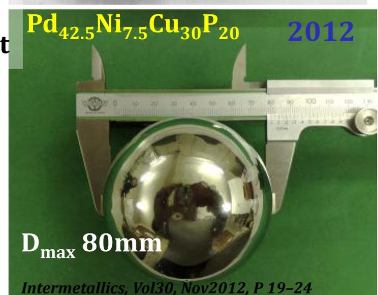
Starting in the late 1980s, the RSP group at Tohoku University in Sendai, Japan, has systematically investigated the glass-forming ability (GFA) of different alloy systems and was able to produce bulk glassy alloys in some of the systems at solidification rates of  $10^3 \text{ K s}^{-1}$  or lower. A brief account of the development of BMGs at Tohoku University is described below.
