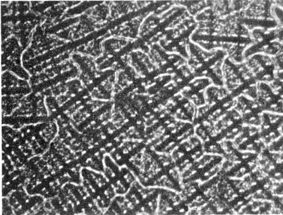
Fig. 5.44. Distribution of Cu in an Al-4.5% Cu alloy
