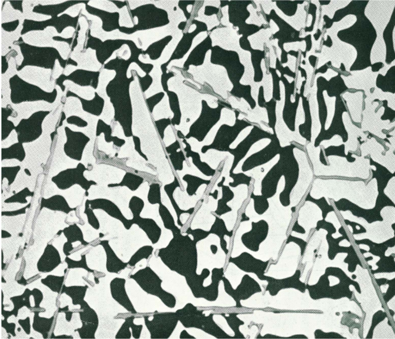
Microstructure of the ternary eutectic in the Al-Cu-Si system. \alpha light, \theta dark, Si grey, (x 900) 32
