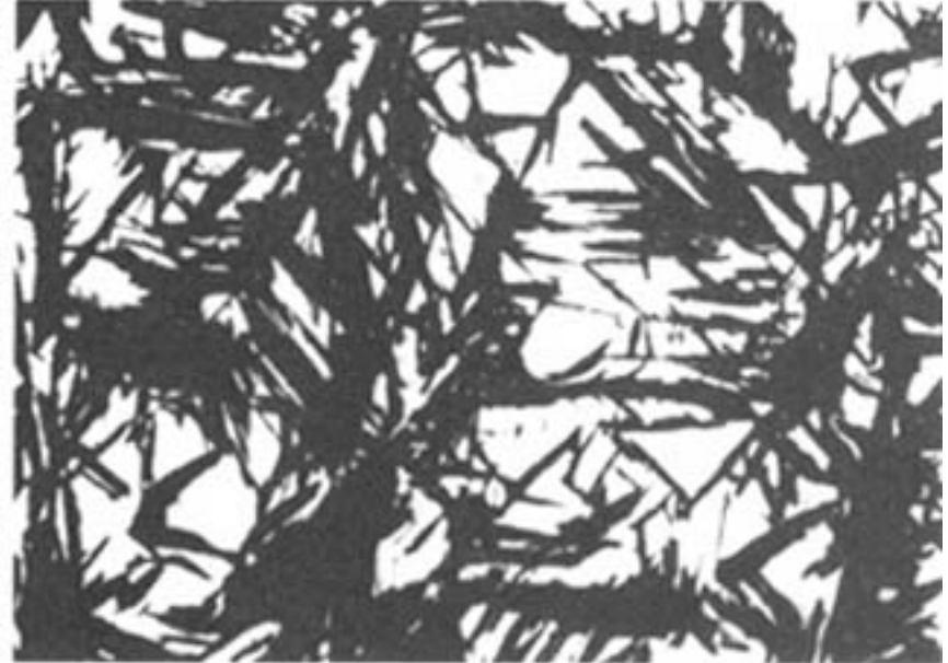
"Needle like" Structure of martensite
