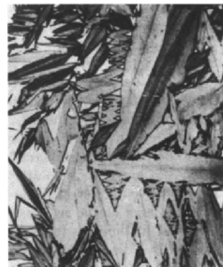
(e) Fe-Ni (plate, some isothermal growth)
