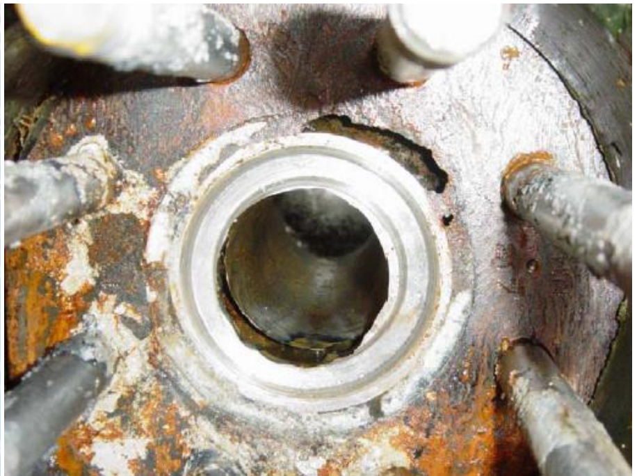
Tree failure (Sand erosion damage)
