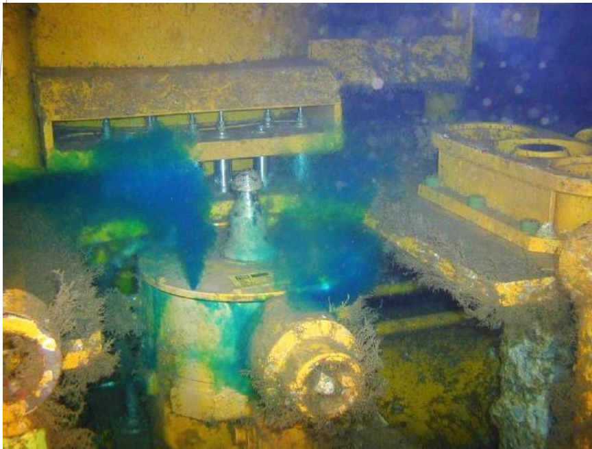
Refraction patterns caused by leaking fluid
