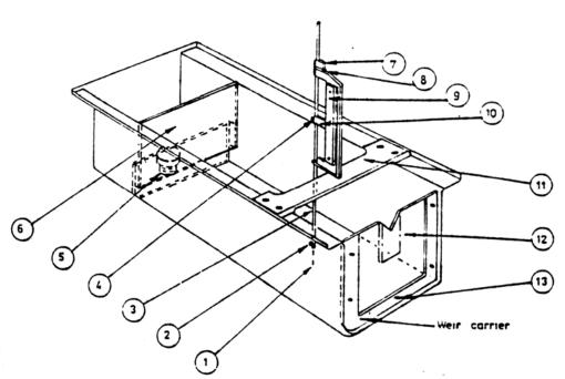
①Point ②Screw C ③Sliding mast ④Screw B ⑤Deliver nozzle ⑥Stilling baffle ⑦Screw A ⑧Fine adjustment nut ⑨Scale ⑩Vernier ⑪Instrument carrier ②Weir plate ⑬Thumb nuts
