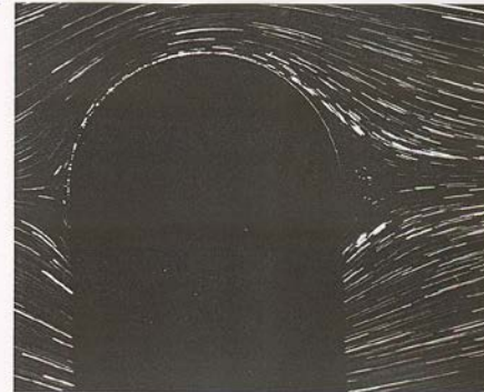
25. Sphere at R=9.8 . Here too, with wall effects negligible, the streamline pattern is distinctly asymmetric, in contrast to the creeping flow of figure 8. The fluid is evidently moving very slowly at the rear, making it difficult to estimate the onset of separation. The flow is presumably attached here, because separation is believed to begin above R=20 . Streamlines are shown by magnesium cuttings illuminated in water. Photograph by Madeleine Costanceau and Michele Foyard
