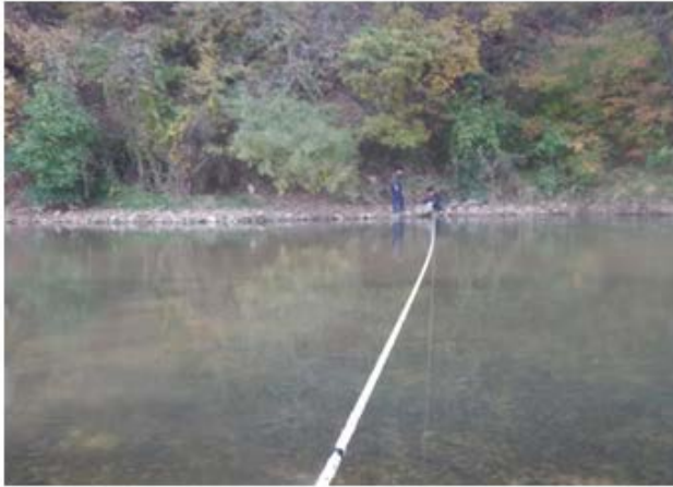
a) Installation of tag line
