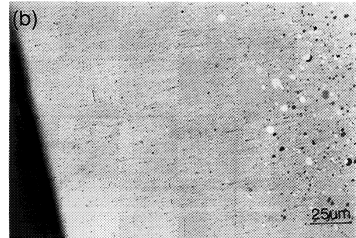
Fig. 4 Optical micrographs taken from the regions (a and b) in the transverse cross section of the cast Zr_{60}Al_{10}Ni_{10}Cu_{15}Pd_5 alloy with the wedge shape of \theta=12.5 degrees.
