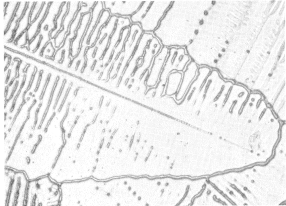
Fig. 5.45. Segregation in Al-Cu alloy
