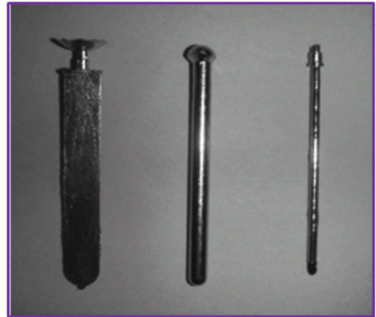
Fig. 6. Photograph of the as-cast specimens of (from left to right): (a) suction cast 12X1X~70 mm 3 plate, (b) drop cast 6.4X~70 mm 2 cylinder, (c) suction cast 3 mm diamX~70 mm cylinder.
