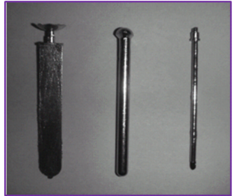
Fig. 6. Photograph of the as-cast specimens of (from left to right): (a) suction cast 12 \times 1 \times 70 mm 3 plate, (b) drop cast 6.4 \times 70 mm 2 cylinder, (c) suction cast 3 mm diam \times 70 mm cylinder.
