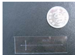
Microchip by direct machining
