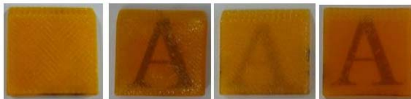
(a) Raw Material T=0,2% (b) Temperature(180°C) T=8,4% (c) Acryl T=1,8% (d) Acryl+Sanding T=22,4%
