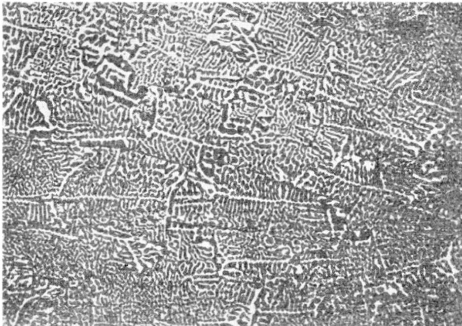
Fig. 6.25. “Chinese script” structure in Bi-Sn eutectic alloy
