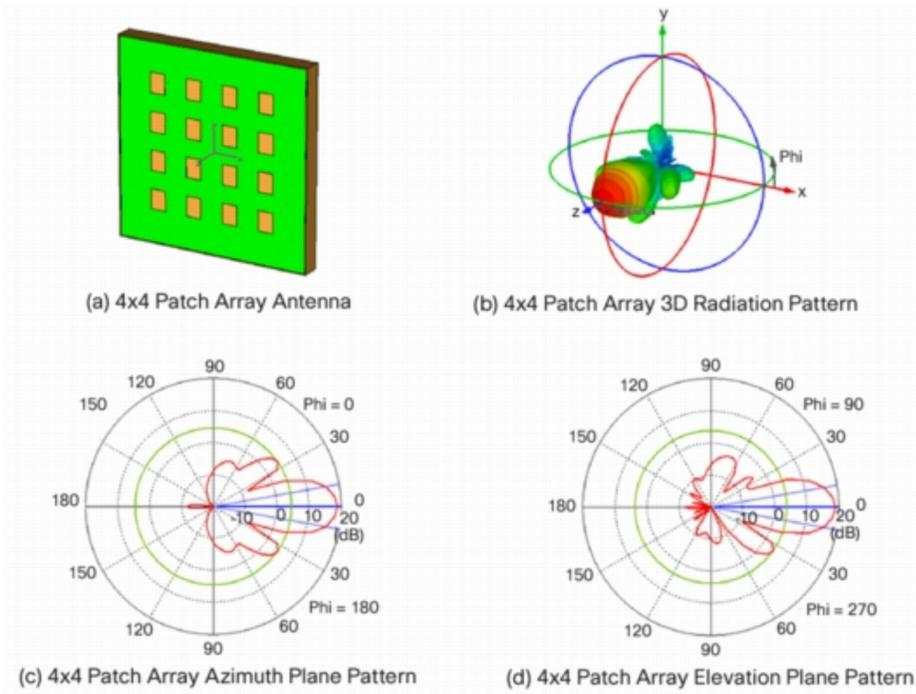
**Patch array antenna = 18 (dBi)**
