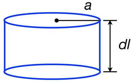
$$\eta_r = \frac{P_r}{P_r + P_l} = \frac{R_r}{R_r + R_l} = \frac{1}{1 + R_l/R_r} \quad \text{where } R_l = R_s \left( \frac{dl}{2\pi a} \right)$$
