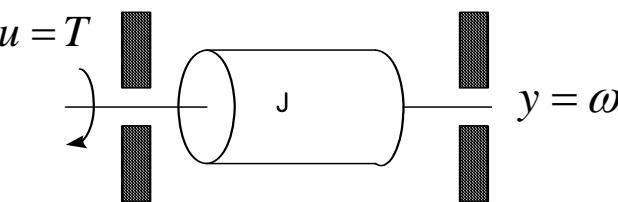
$$J\dot{\omega} + b\omega = T \quad \frac{Y}{U} = \frac{\omega}{T} = \frac{1}{Js + b}$$
