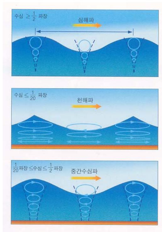
Water particle motions in deep, shallow, and intermediate-depth waters
