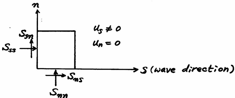
$$[S] = \begin{bmatrix} S_{ss} & S_{sn} \\ S_{ns} & S_{nn} \end{bmatrix} \quad \begin{array}{l} \text{1st subscript = plane} \\ \text{2nd subscript = direction} \end{array}$$
