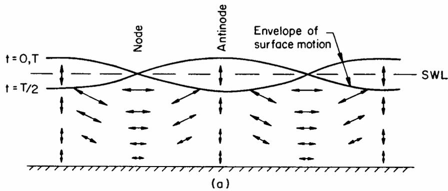
Under the pure standing wave, at  $t = 0$  or  $T/2$ , the water particle motion stops for an instant so that only potential energy exists, while at  $t = T/4$  or  $3T/4$ , the water surface becomes flat so that only kinetic energy exists. Also,  $w = 0$  at nodes, while  $u = 0$  at antinodes.
