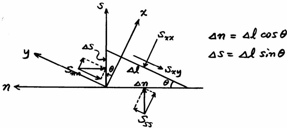
$$\Delta l S_{xx} = S_{ss} \cos \theta \Delta n + S_{nn} \sin \theta \Delta s = S_{ss} \cos^2 \theta \Delta l + S_{nn} \sin^2 \theta \Delta l$$
