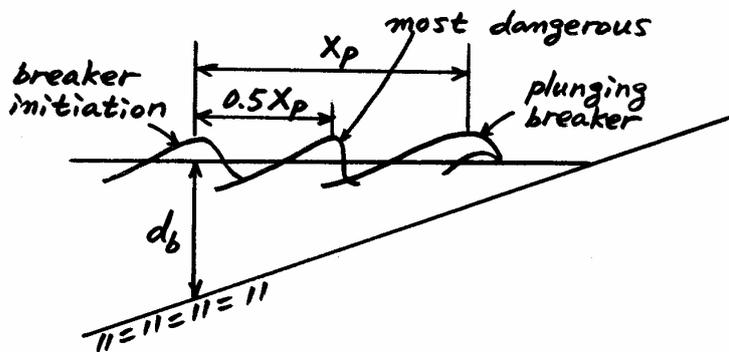
The most dangerous point is about  $0.5X_p$  from the breaker initiation point, where  $X_p$  is the distance from breaker initiation to plunging point. Therefore, it is needed to design the structure for the waves breaking at  $0.5X_p$  seaward of the structure. For plane slope,
