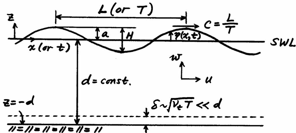
$d$  = water depth;  $L$  = wavelength;  $T$  = wave period;  $C$  = wave celerity (speed);
