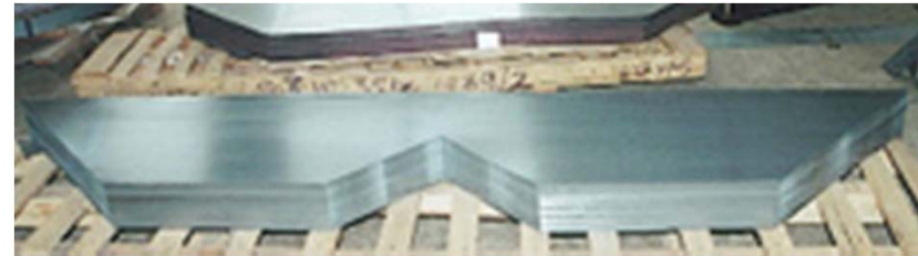
Stacked transformer core
