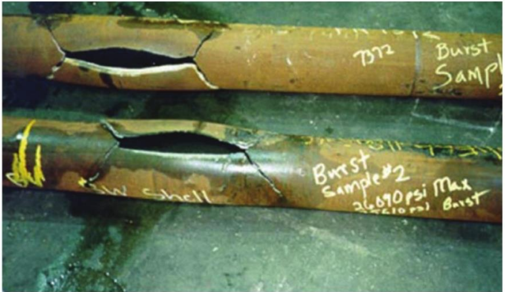
Figure A.2—Brittle Burst Sample
