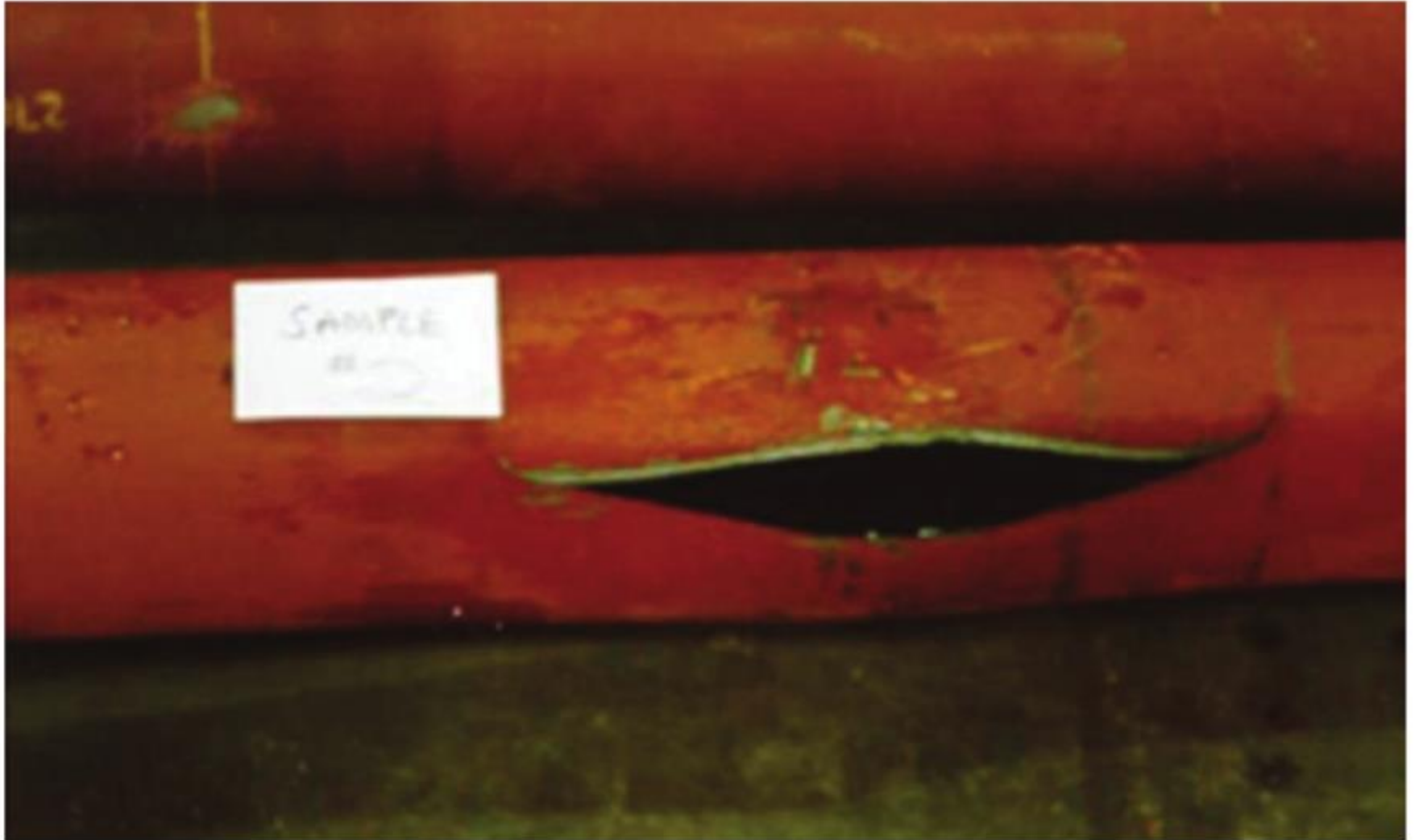
Figure A.1—Ductile Burst Sample
