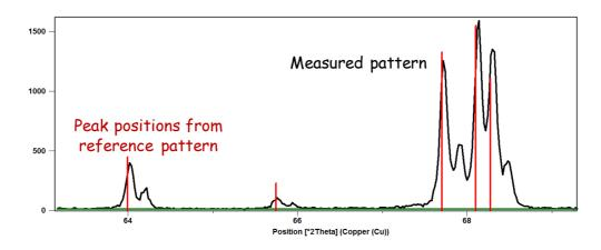
> A small amount of mismatch in peak position and intensity is acceptable experimental error
