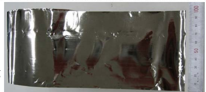
Fig. Photograph of the melt-spun Ni-Nb-Zr-Co amorphous alloy of 100mm in width.
