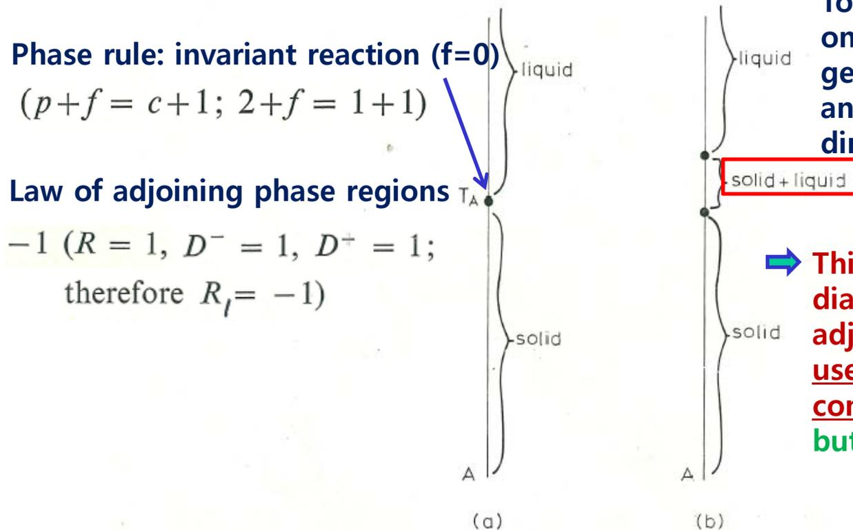
To overcome this situation, one regards the point  $T_A$  as a degenerate (liquid+solid) phase region and one replaces the missing dimension to give the diagram.
