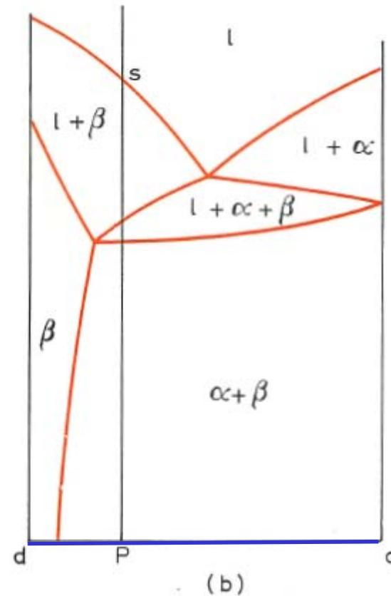
Fig. 261. Freezing of quaternary alloy P illustrated by reference to the polythermal projection of Fig. 255.
