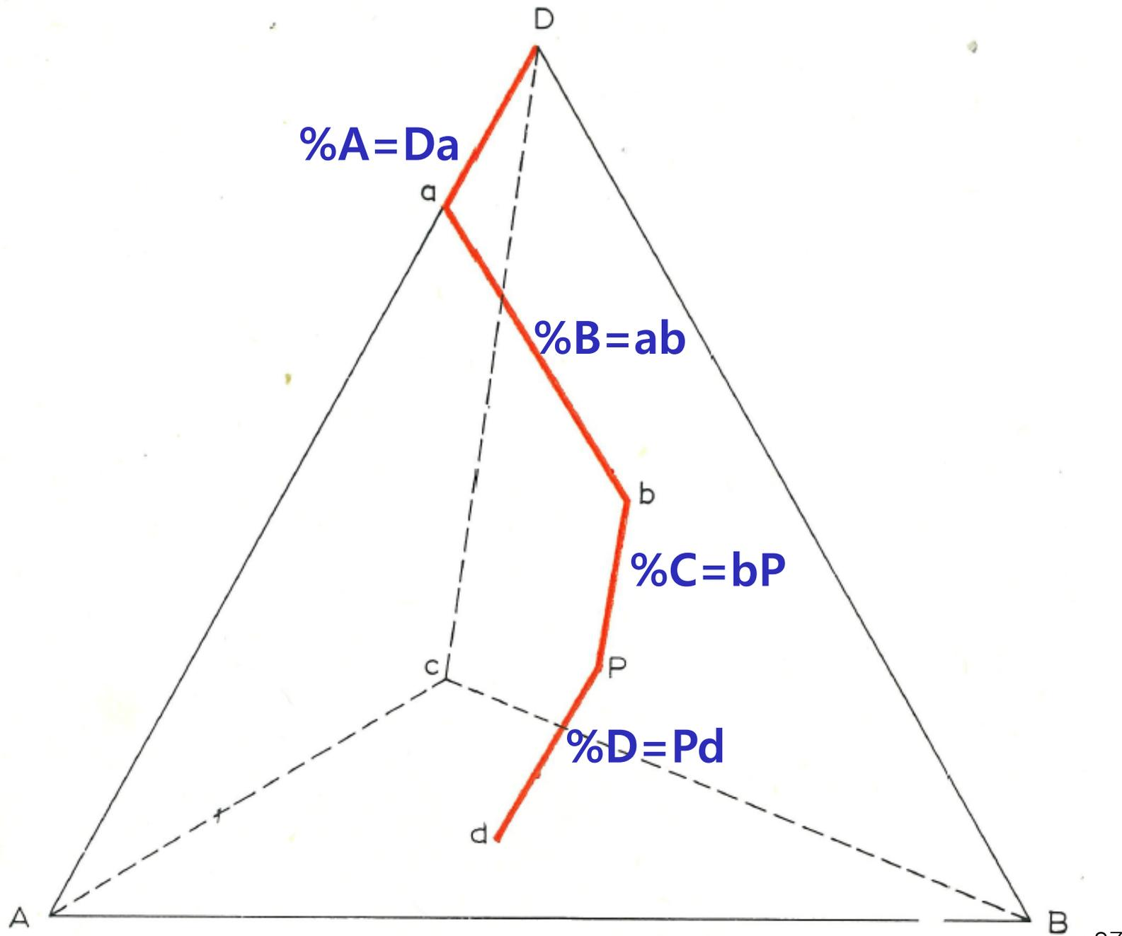
Fig. 248. Plotting of alloy compositions in quaternary systems.
