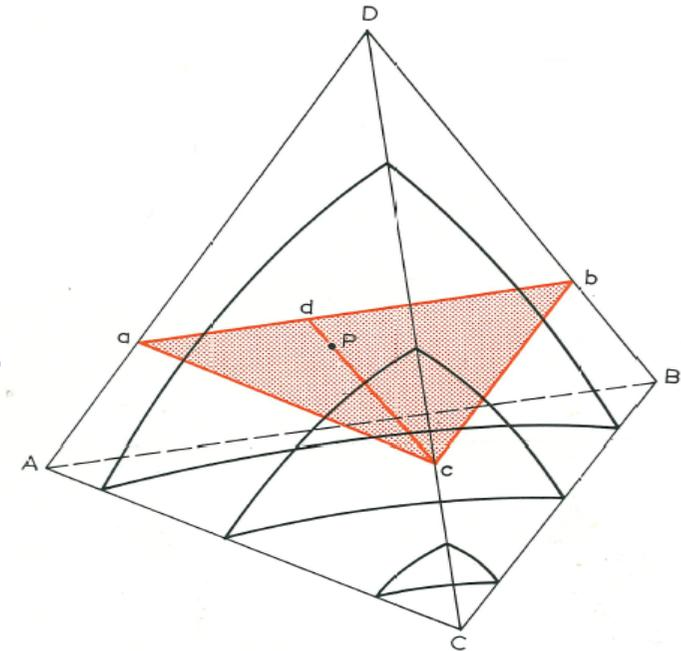
Fig. 258. Position of alloy *P* on plane *abc*.
