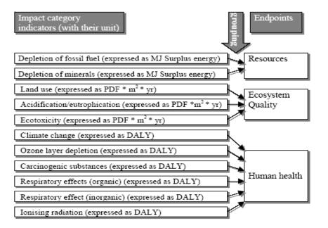
Illustration of the grouping option on the Eco-indicator99 method. This procedure allows to reduce the number of impact categories to just three instead of 11 without subjective weighting
