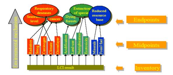
General overview of the structure of an impact assessment method. The LCI results are characterised to produce a number of impact category indicators. According to ISO, one must document the environmental relevance of each indicator by describing the link to the endpoints. Endpoints can be selected by the practitioner, as long as the reasons for including or excluding endpoints are clearly documented.
