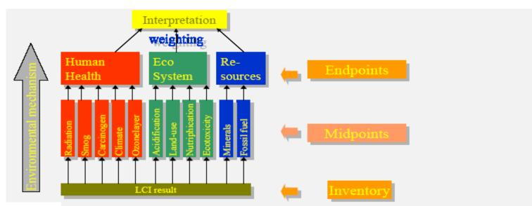
Schematic overview of the methodology proposed by Goedkoop & Spriensma. The environmental models for each impact category are extended up to endpoint level, as the impact category indicators that relate to the same endpoint have a common unit, these indicators can be added. In the case of ecotoxicity, the endpoint is Ecosystem Quality, expressed as Potential Disappeared Fraction of plants
