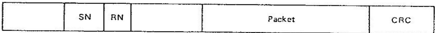
Figure 2.20 The header of a frame contains a field carrying the sequence number, SN , of the packet being transmitted. If piggybacking is being used, it also contains a field carrying the request number, RN , of the next packet awaited in the opposite direction.
