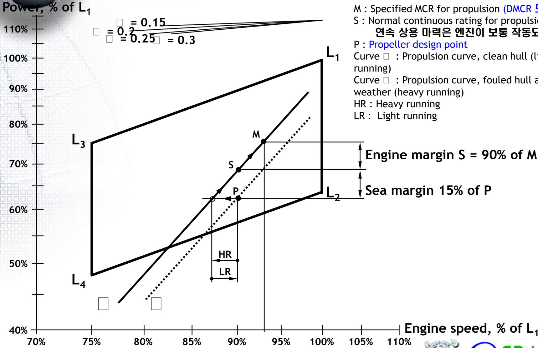
M : Specified MCR for propulsion (DMCR 또는 MCR)
