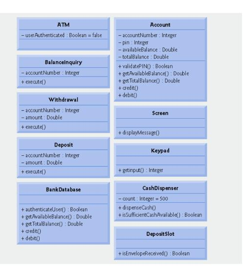
Fig. 9.20 | Class diagram with visibility markers.
