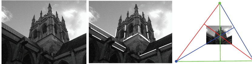
Fig. 7.20. For the case that image skew is zero and the aspect ratio unity the principal point is the orthocentre of an orthogonal triad of vanishing points. (a) Original image. (b) Three sets of parallel lines in the scene, with each set having direction orthogonal to the others. (c) The principal point is the orthocentre of the triangle with the vanishing points as vertices.
