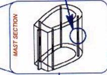
Optical fibre sensors are embedded into structure and are so small that they form part of the laminate structure
