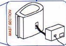
Optical signal splitting at fibre exit from laminate
