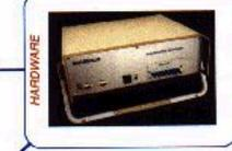
Optical Fibre Strain Sensor System (OFSS) which acquires and initially processes data
