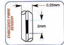
Bragg grating strain sensor produced by internally modifying optical fibre with UV laser
